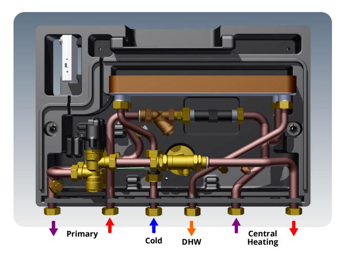
All connections are bottom entry, with a first fix kit as an optional extra. The fixing kit spaces the unit 50mm from the wall to allow pipes to be run up the back.
